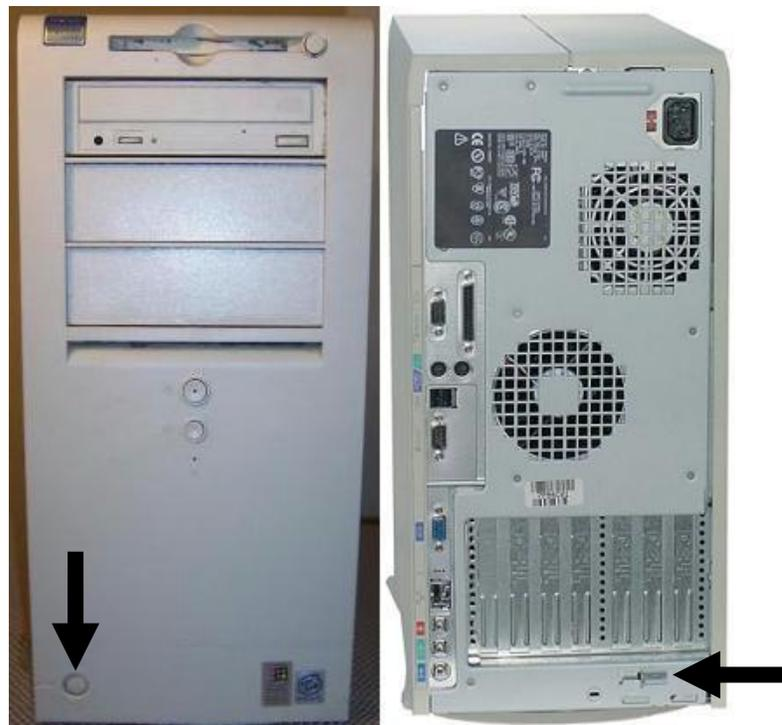
Next, press the small plastic button on the front of the case at the bottom to release the one side of the PC case. The arrow in the above picture shows where the button is on the front of the PC. The case can be lifted up and then removed. Here is a visual from Dell's website which illustrates how the case is removed.
